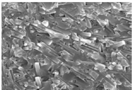
Ultra-strong whiskers provide increased fracture toughness and notch wear resistance
