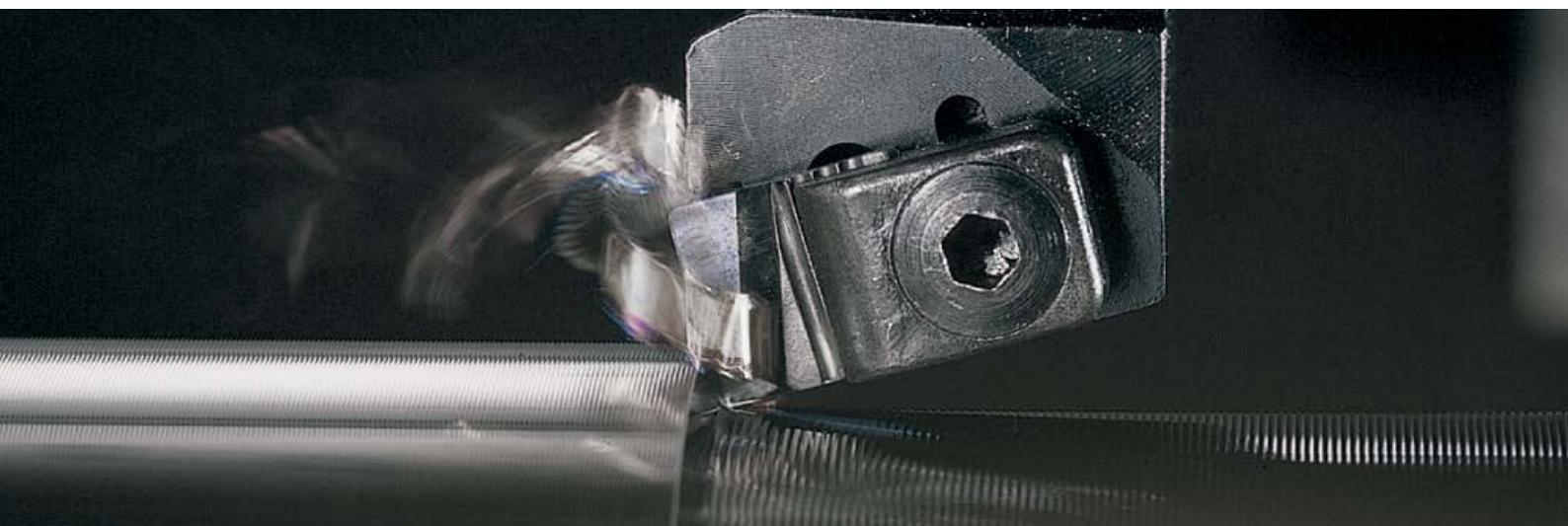
**Whisker reinforced ceramic for greater fracture resistance**
