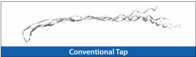
■ Chip generated in 40m/min
